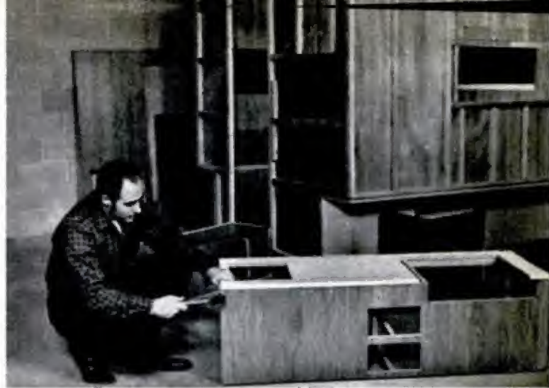
INTERIOR PARTITIONS are also precut and pre-finished. Camper can be assembled in about 50 hours
